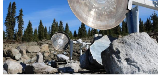
Giant diamond saws cut the boulders to enable better examination of the material.
